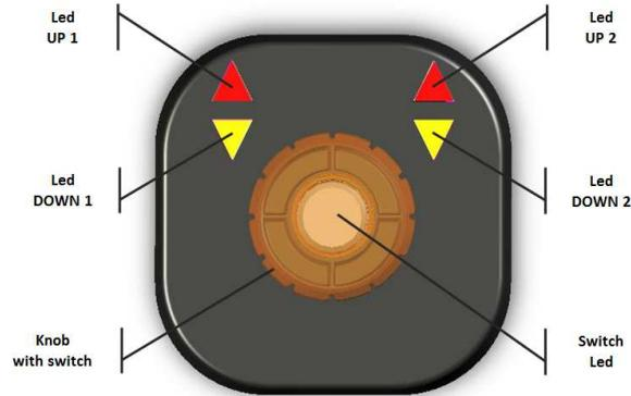
The multifunction Easy Lift's knob allows to select and activate the desired programs in a simple and intuitive way. The device has also a switch and a signalling led.
